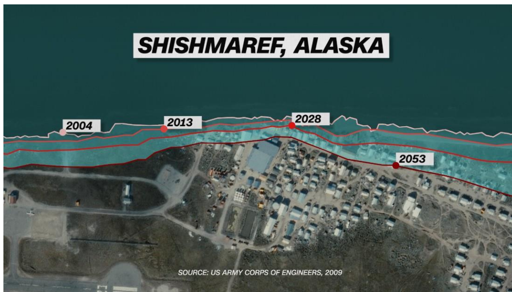
Source: U.S. Army Corps of Engineers, 2009.
